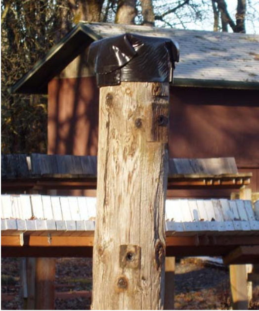
Figure III-8. Example of a capped pole (Osrose Pole Topper) used to assess the effects of capping on wood moisture content.
