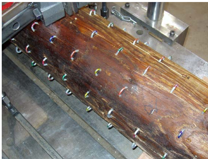
Figure III-11. Example of a pole containing rows of ground wire staples driven into the surface.
