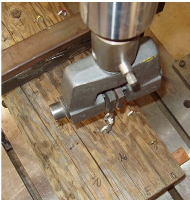
Figure III-10. Example of a ground wire staple being driven into a Douglas-fir pole section.
